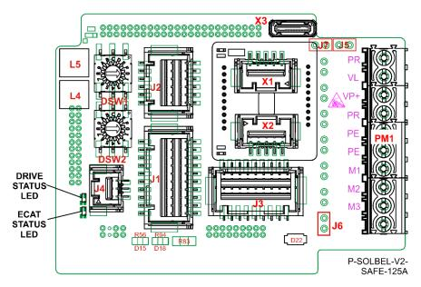
Figure 4: Platinum Solo Bell Board Indicator Labelling
