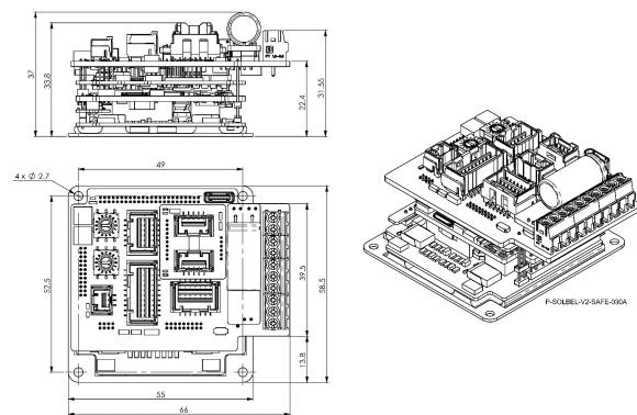
Figure 46: Platinum Solo Bell with Safe IO Board
