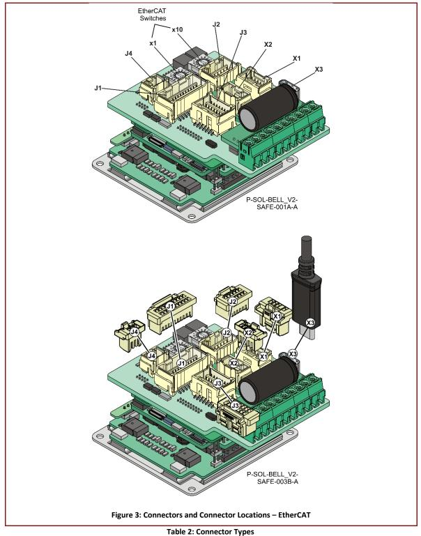
The pinouts in Chapter 8: Wiring describe the function of each pin in the Platinum Solo Bell connectors that are listed in Table 2.
