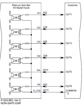
Figure 32: Regular Digital Input 5V Logic Connection Diagram
