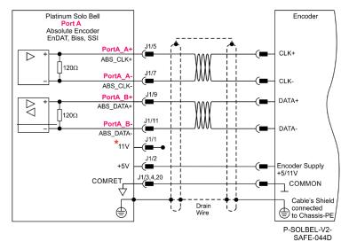
Figure 17: Absolute Serial Encoder – Recommended Connection Diagram for EnDat, Biss, SSI
