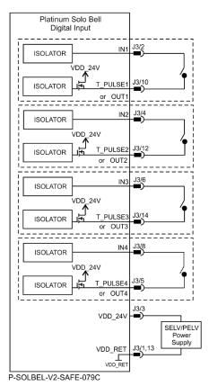
Figure 27: Digital input with Test Pulse
