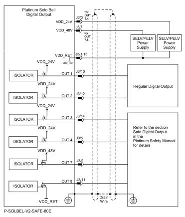
Figure 30: Safe Digital Outputs for Option L Configuration
