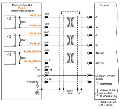
Figure 19: Port B Incremental Encoder Input – Recommended Connection Diagram
