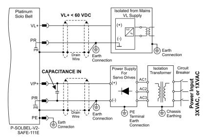
Figure 13: Power Supply Connection Diagram for Safety Configuration
