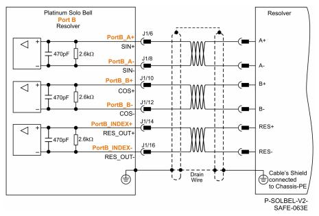
Figure 21: Port B – Resolver Connection Diagram
