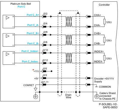
Figure 25: Emulated Encoder Differential Output – Recommended Connection Diagram
