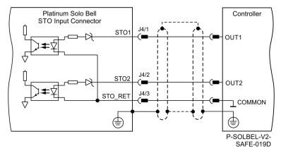
Figure 14: STO Type Connection – PLC Source Option
