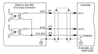
Figure 15: STO Input Connection – TTL Option
