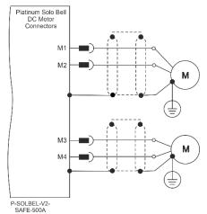
Figure 12: Two Motor Power Connection Diagram
