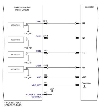
Figure 37: Regular Digital Output Connection Diagram – PLC Sink Option
