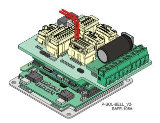
Figure 6: Inserting a wire/pin to the Female CON CLIK-MATE Connector
