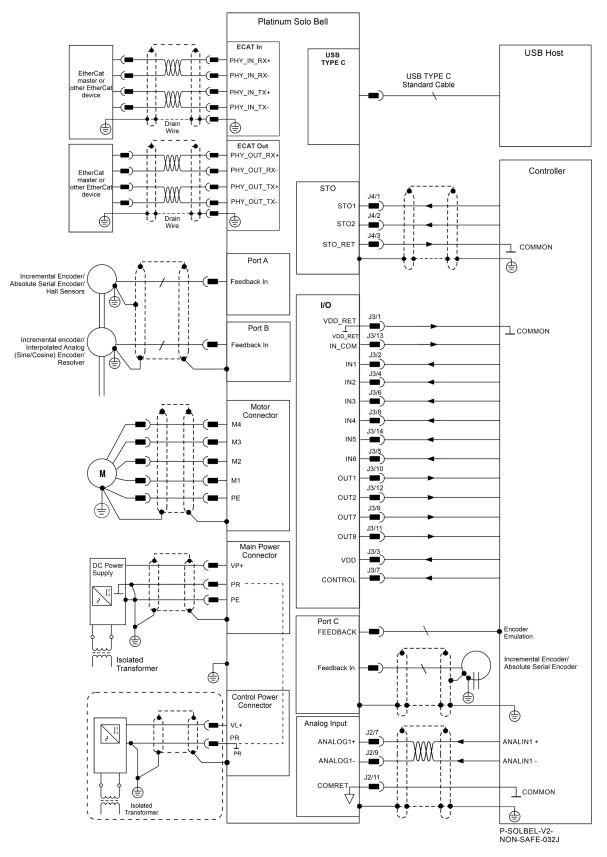
Figure 8: The Platinum Solo Bell without Safe IO, Connection Diagram – EtherCAT
