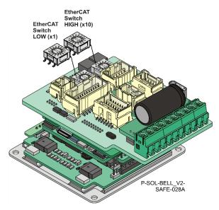
Figure 44: EtherCAT Address Switches
