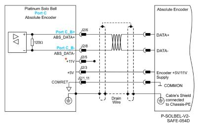
Figure 24: Absolute Serial Encoder – Recommended Connection Diagram for Pansonic, Tamagawai, Sanyo-Danki
