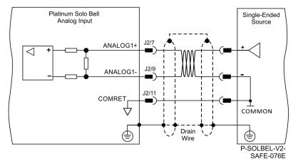
Figure 38: Differential Analog Input
