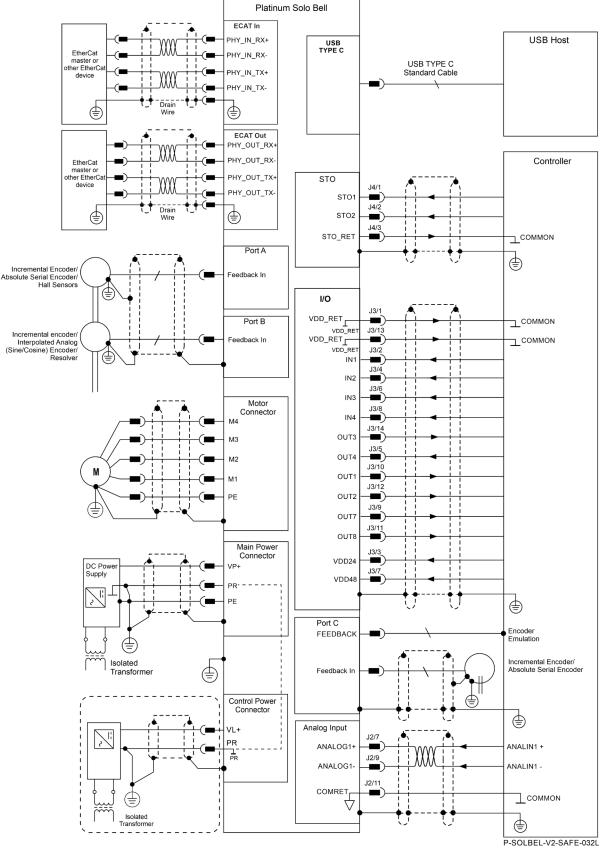
Figure 7: The Platinum Solo Bell with Safe IO, Connection Diagram – EtherCAT
