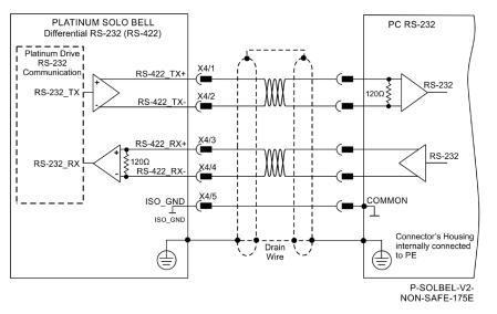
Figure 39: Differential RS-232 Communication Example
