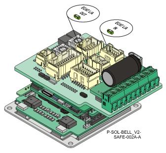
Figure 43: Ethernet Connector LEDs
