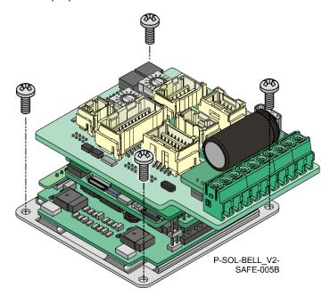
Figure 1: Mounting the Platinum Solo Bell
