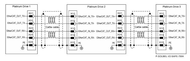
Figure 41: EtherCAT Connection Schematic Diagram
