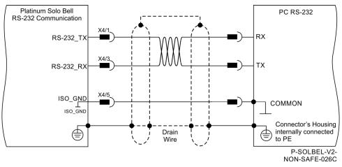
Figure 40: RS-232 Connection Diagram
