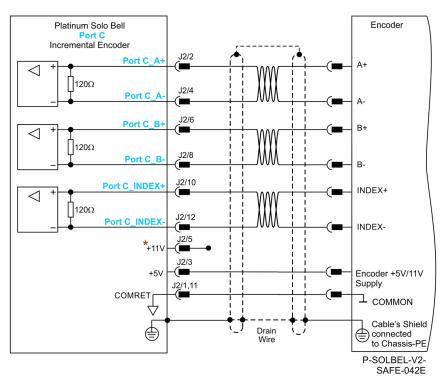
Figure 22: Port C Incremental Encoder Input – Recommended Connection Diagram
