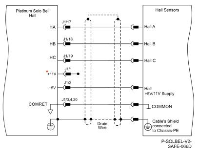
Figure 26: Hall Sensors Connection Diagram
