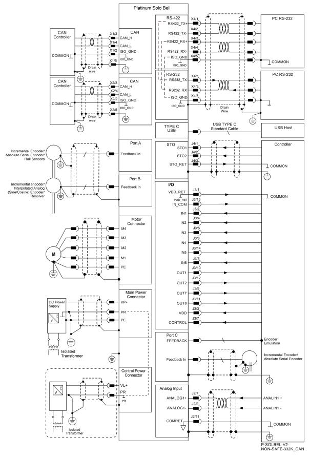
Figure 9: The Platinum Solo Bell Connection Diagram - CAN
