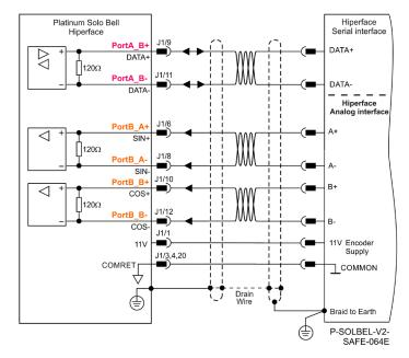
Figure 18: Absolute Serial Encoder – Recommended Connection Diagram for Stegmann Hiperface
