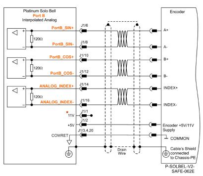
Figure 20: Port B - Interpolated Analog Encoder Connection Diagram
