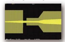
Built-in Low Voltage Ride Through (LVRT) mode can simulate the grid in abnormal conditions The settings include voltage, frequency, drop voltage, recovery voltage, rise time and hold time to simulate various conditions.
