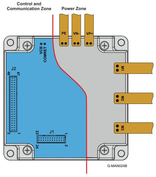
Figure 3: Gold Mandolin Power Conductors PCB layout
