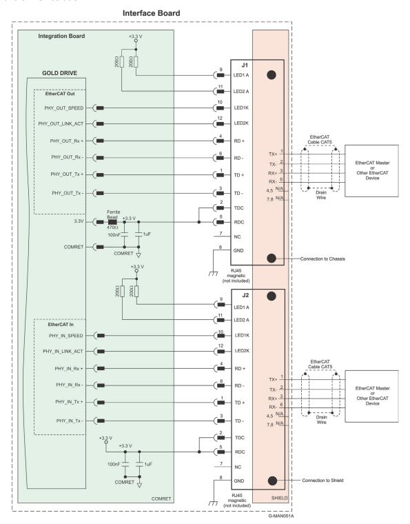
Figure 28: EtherCAT Connection Schematic with Diagram Sign of 3.3V
