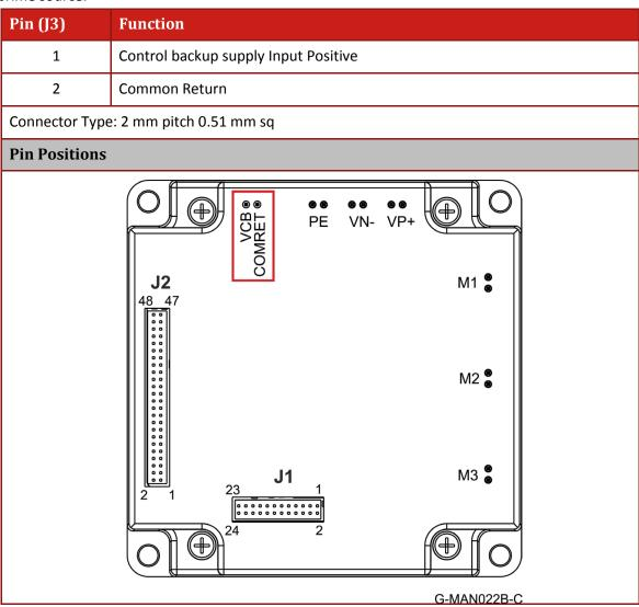
**Table 4: 24 VDC Control Supply Pins and Polarity**
