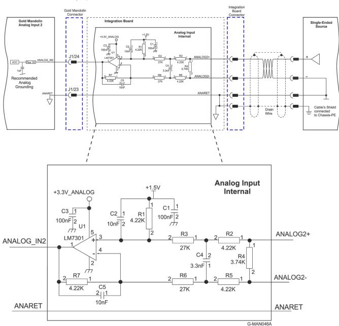
Figure 25: Analog Input 2 Example
