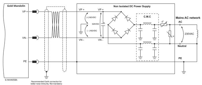
Figure 9: Non-Isolated Single-Phase Connection Topology
