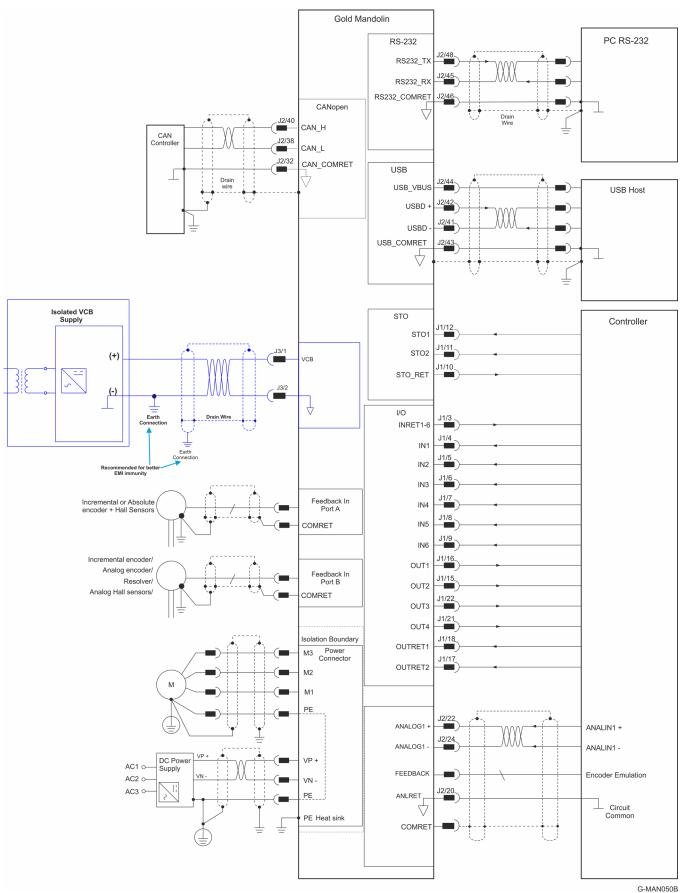
Figure 5: Gold Mandolin Connection Diagram for CAN
