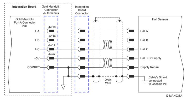
**Figure 16: Hall Sensors Connection Diagram**
