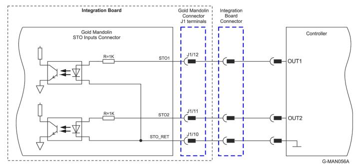
Figure 32: STO Input Connection - TTL Option
