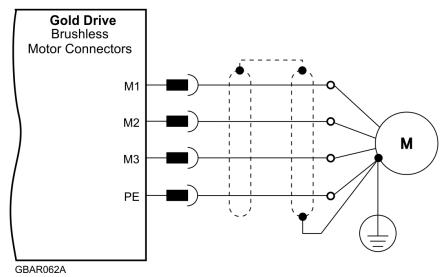
**Figure 6: Brushless Motor Power Connection Diagram**
