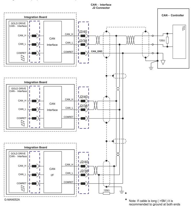
**Figure 29: CANbus Connections**
