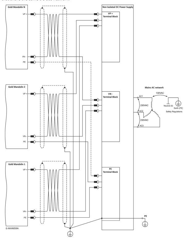
Figure 10: Non-Isolated Three-Phase Multiple Connection Topology
