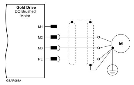
**Figure 7: Brushed Motor Power Connection Diagram**
