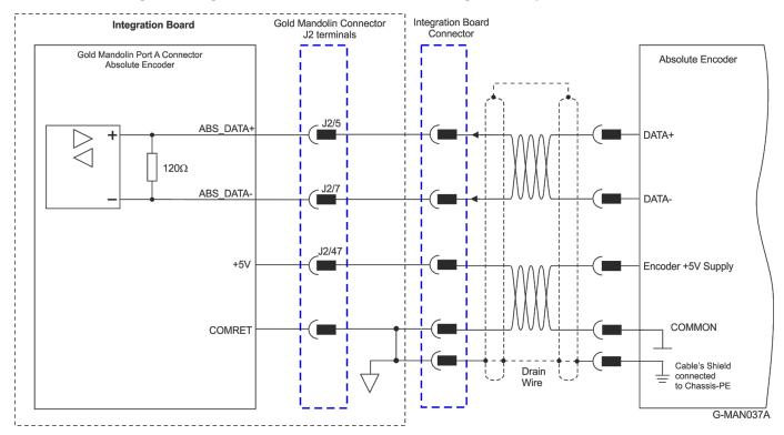
Figure 18: Absolute Serial Encoder – Recommended Connection Diagram for Pansonic, Tamgawai, Sanyo-Danki
