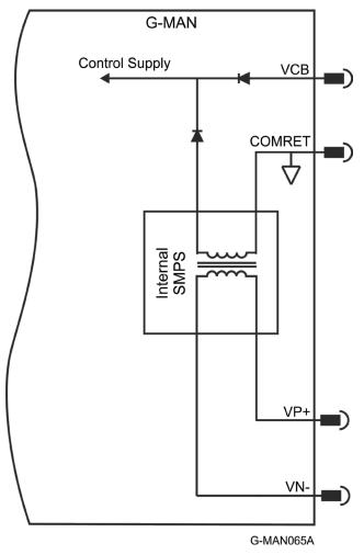
Figure 12: Switch-mode Power Supply
