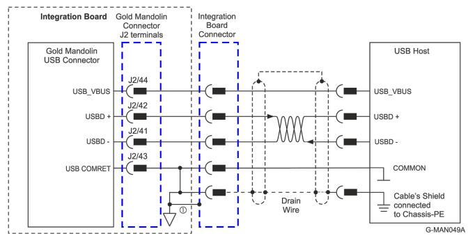
Figure 27: USB Network Diagram
