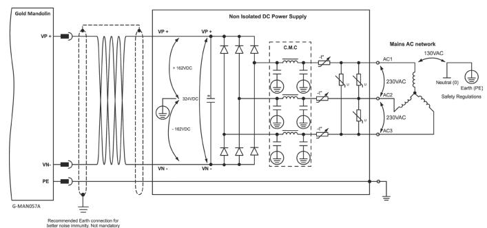
Figure 8: Non-Isolated Three-Phase Connection Topology
