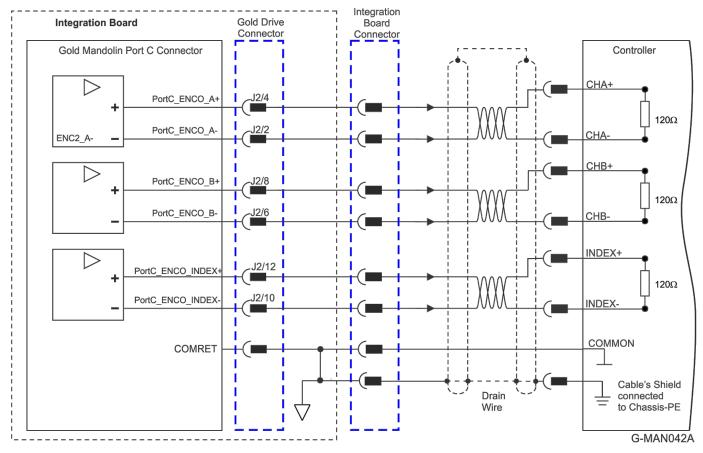
Figure 23: Emulated Encoder Differential Output – Recommended Connection Diagram
