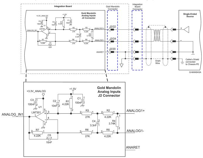
Figure 24: Analog Input with Differential ±10 V
