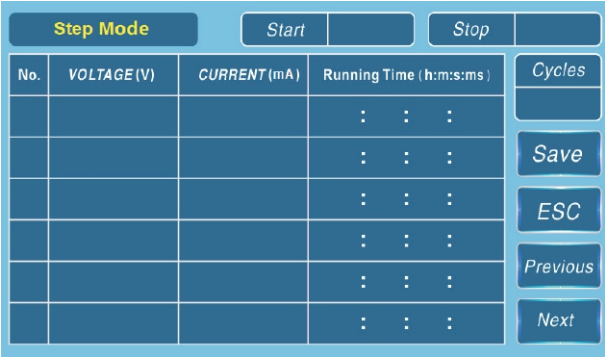
The step setting page can set the required frequency, voltage, running time, initial step, end step and cycle times.
